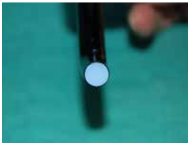
FIGURE 9A The examination of two light guides by holding them up to daylight. The blotching of the surface of the guide on the right indicates damaged fibres
