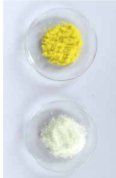
FIGURE 6 Note the different in colour between the yellow camphorquinone on top and the white Lucirin TPO below
