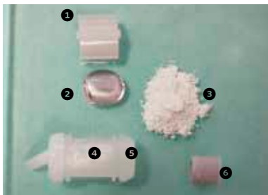
FIGURE 9 The contents of a capsule: 1. Plastic clip 2. Pillow 3. Powder 4. Access hole 5. Outer casing 6. Plunger
