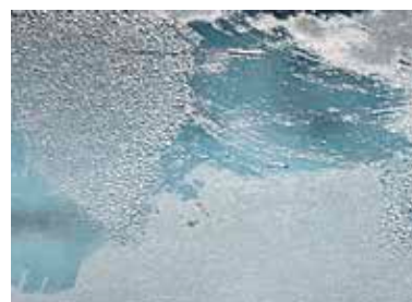
FIGURE 4 Drops of water condensing on a chilled glass slab. Incorporation of this water into the powder/liquid mix will affect the final properties of the cement
