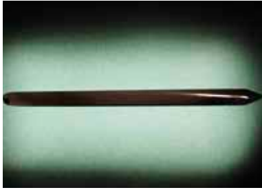
FIGURE 7 An agate spatula which should be used to hand mix glass ionomer cements
